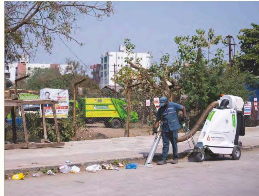
Pavements cleaning with the help of Electric Glutton
